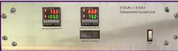
Remote temperature control unit
